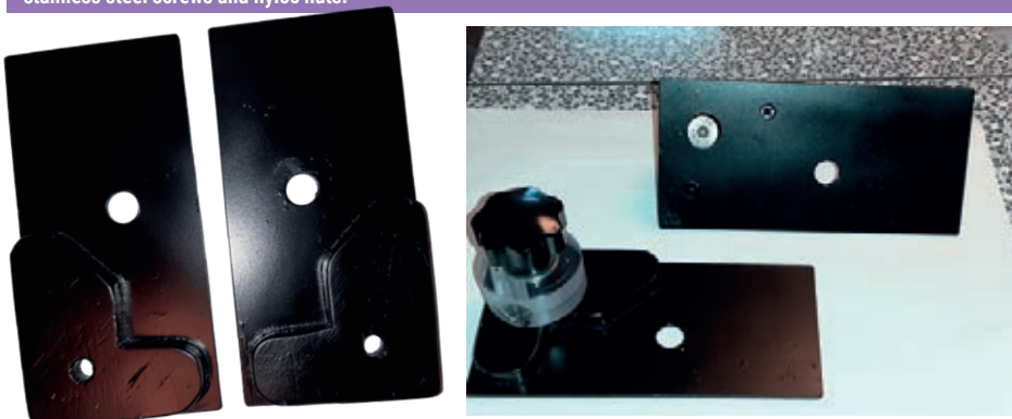
2. A good line for the wind deflector seemed to be slightly forward of the seat belt reel mounts, and this also suggested a means of fixing. Mounting plates were made from 2mm aluminium sheet and 10mm ply.
