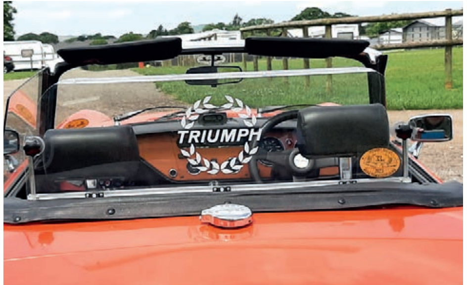
7. The braces were fastened to the hood fixing brackets. The final finishing touch was a Triumph laurel leaf transfer.
