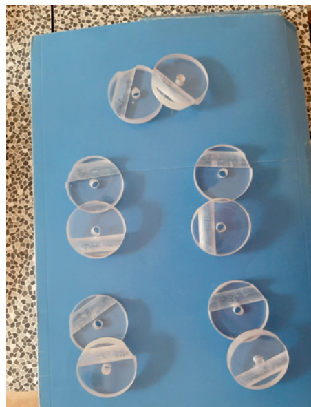
4. Tube fixing clamps were made from 10mm thick polycarbonate discs with a semi-circular groove machined off-centre.
