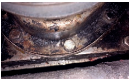
1. The bottom timing cover bolt seeping oil.
