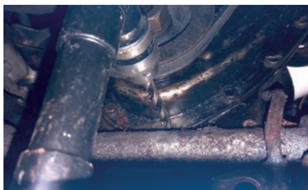
2. Carefully drilling out the stripped thread.
