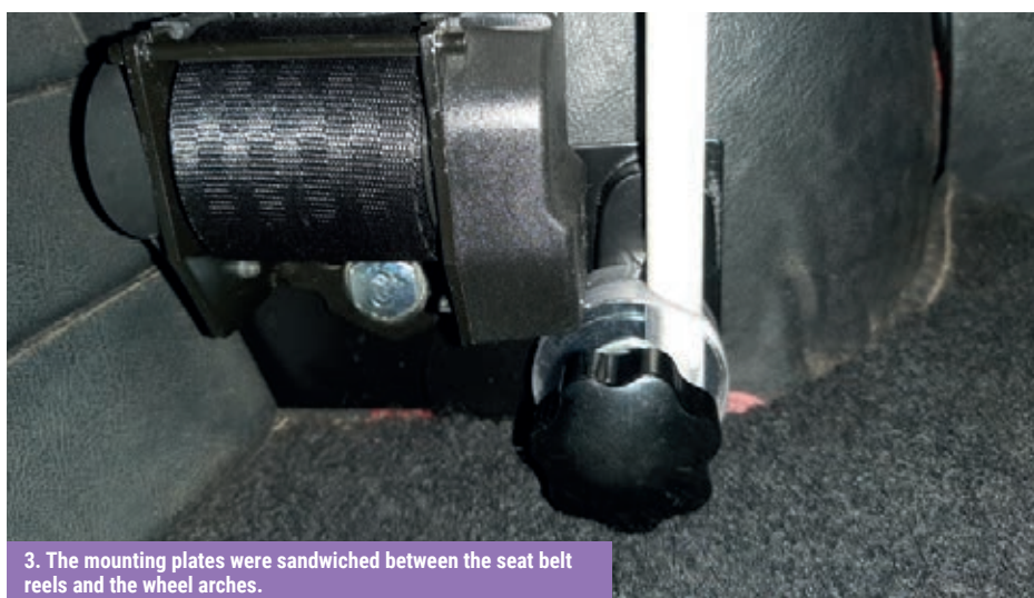
2. A good line for the wind deflector seemed to be slightly forward of the seat belt reel mounts, and this also suggested a means of fixing. Mounting plates were made from 2mm aluminium sheet and 10mm ply.
