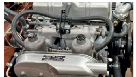
The SU carbs had the bodies bushed to ensure there were no air leaks around the throttle spindle and then fitted with a complete rebuild kit, including conversion away from Waxstat jets.
