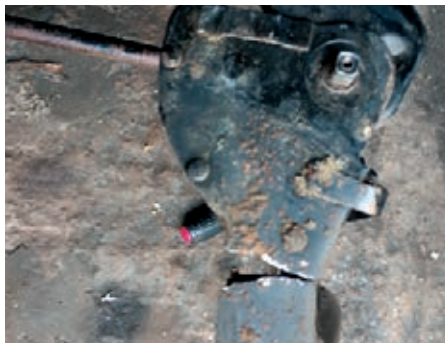
1. A big stress fracture on the driver's seat.
