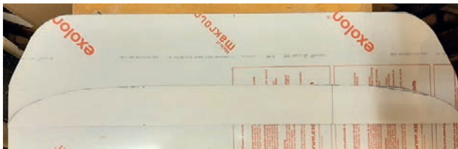
1. Two pieces of 5mm polycarbonate sheet were ordered, cut roughly to shape using a jigsaw and then to final profile using a router and MDF template. The two sections were hinged together using three nylon friction hinges, stainless steel screws and nyloc nuts.
