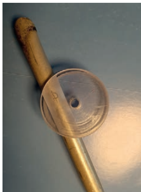
5. These were used in matched pairs to fix the stainless steel tube to the aluminium plates and to the polycarbonate deflector.
