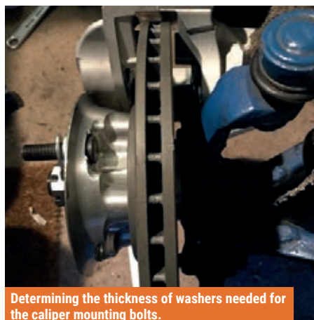
The new brakes assembled – early days as they need to bed in, but the car pulls up well with little effort.
